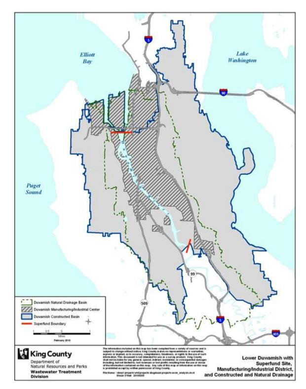
Figure 2: Map of Lower Duwamish River showing Lower Duwamish Waterway Superfund Site, Duwamish Manufacturing and Industrial District (MIC), and constructed and natural drainage.<sup>5</sup>
